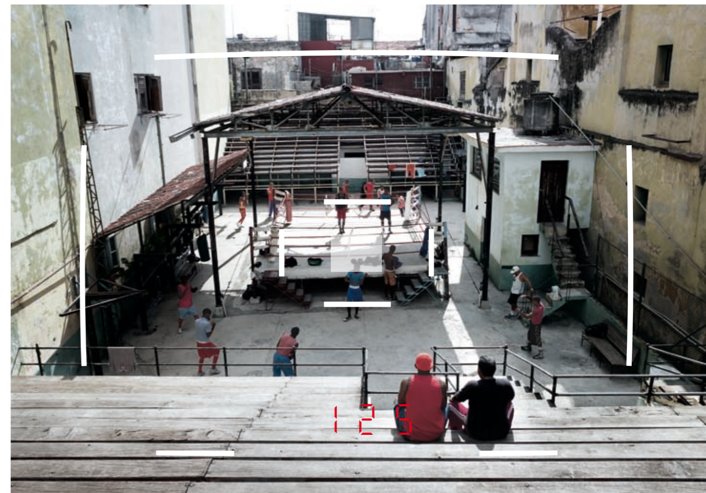
What you see through the viewfinder of an M camera: The inner bright-line frame shows the image boundaries for a 90-mm lens, while the outer frame shows the boundaries for a 28-mm lens. The grey rectangle in the center is the rangefinder focusing area.
